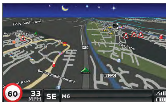
Night view will change both the screen brightness and the map colours.
